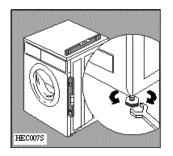
Accurate levelling prevents vibration, noise and displacement of the machine during operation. Never place cardboard, wood or similar materials under the machine to compensate for any unevenness in the floor.
